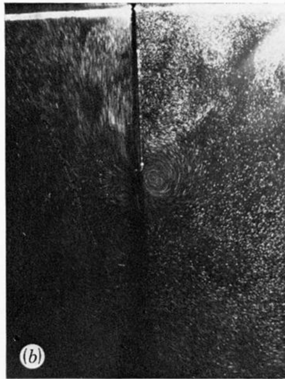
FIGURE 7. Photographic sequence of wave motion interacting with surface piercing plates. Bottom of plate 11 cm below surface. Wave amplitude = 11 mm, wave frequency = 0.83 Hz.
