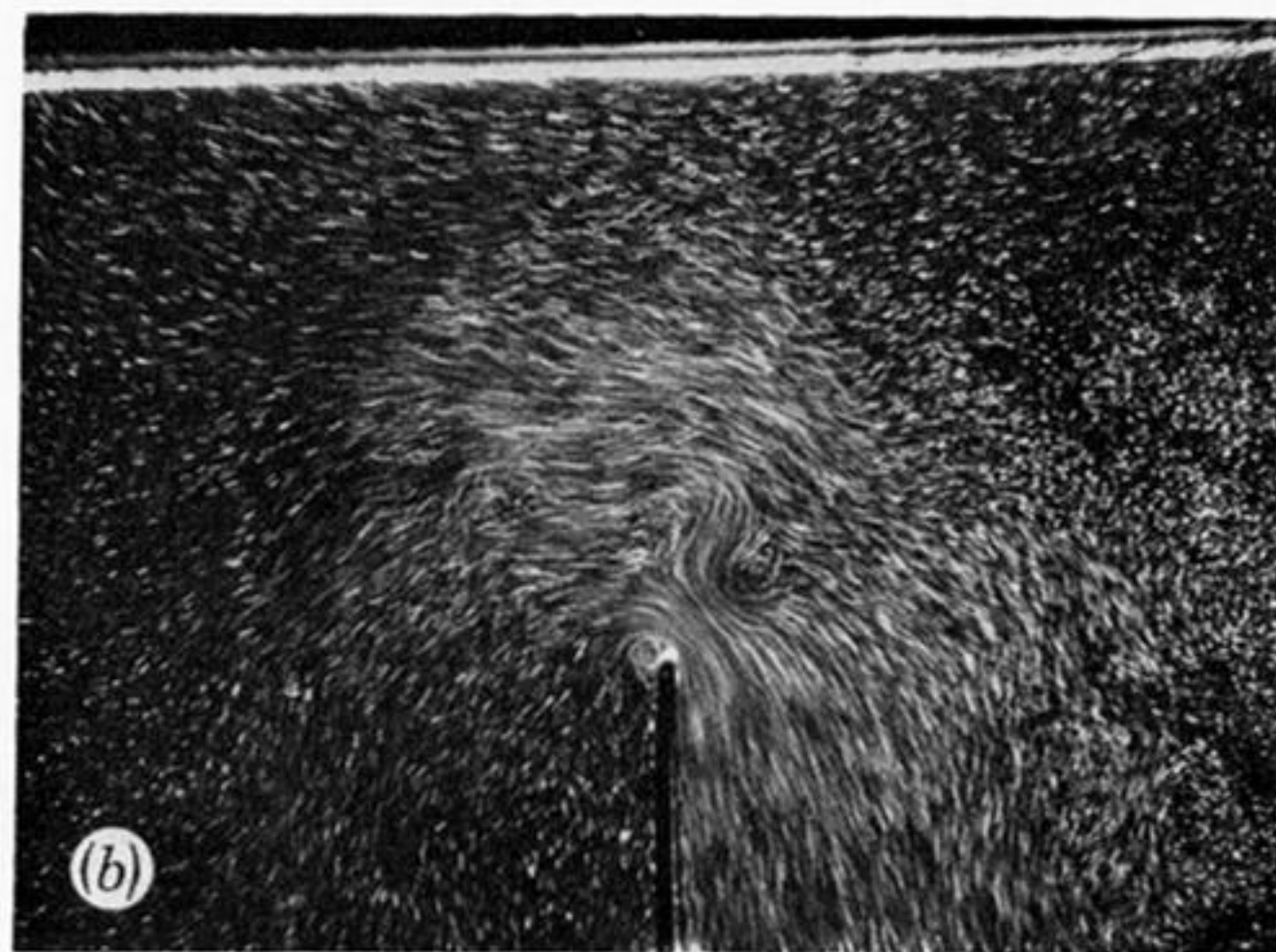
FIGURE 6. Photographic sequence showing the effect of wave amplitude on the intensity of jet eddy pair formation. Wave frequency = 0.83 Hz. Wave amplitude (a) = 2 mm, (b) = 5 mm, and (c) = 11 mm. Other details as figure 4.
